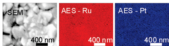
Figure 5. SEM image (left) and AES elemental mapping of Ru and Pt (middle and right), respectively, of sample S4.
